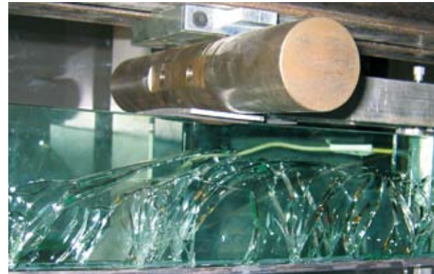
Master thesis project examining the long and short term stiffness of reinforced glass beams. Even after severe cracks in the beams much of the load capacity remained.
