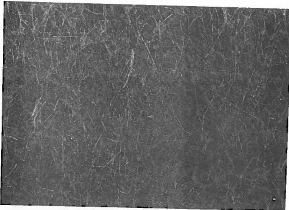
Fig.10 Reinforcing paper of glass-wool fibres (x 10)
