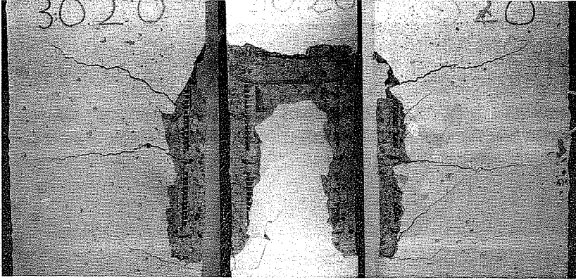
Photo 3.11 Failure of S.B.-specimen No. 30/20.
